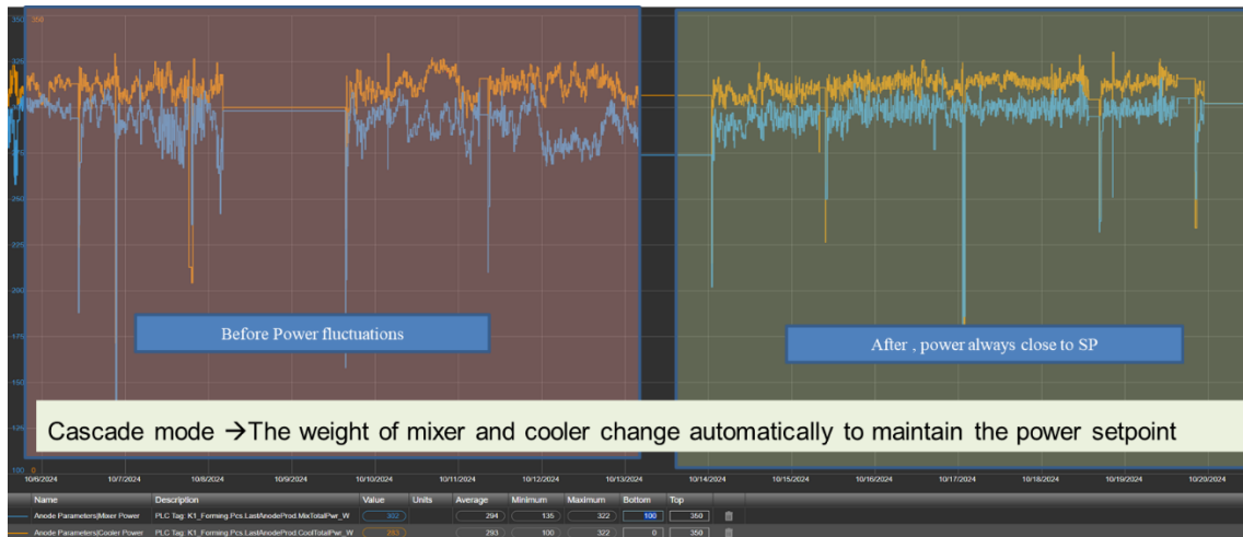
Figure 8. Mixer and cooler PID in cascade mode.
